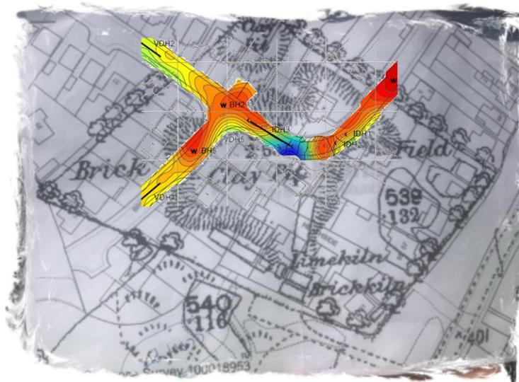
Gravity anomaly surveys measure differences in the mass of the soil below ground and are used to detect both voids and buried structures.
